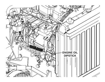
Figure 7-4. Engine Dipstick Location
